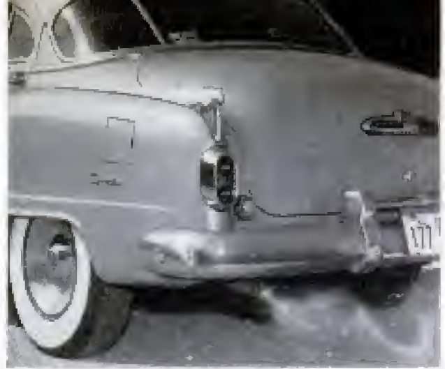
A cloud of blue smoke from the exhaust shows that the car is an oil-burner. Correcting this condition requires a complete engine overhaul which is costly
